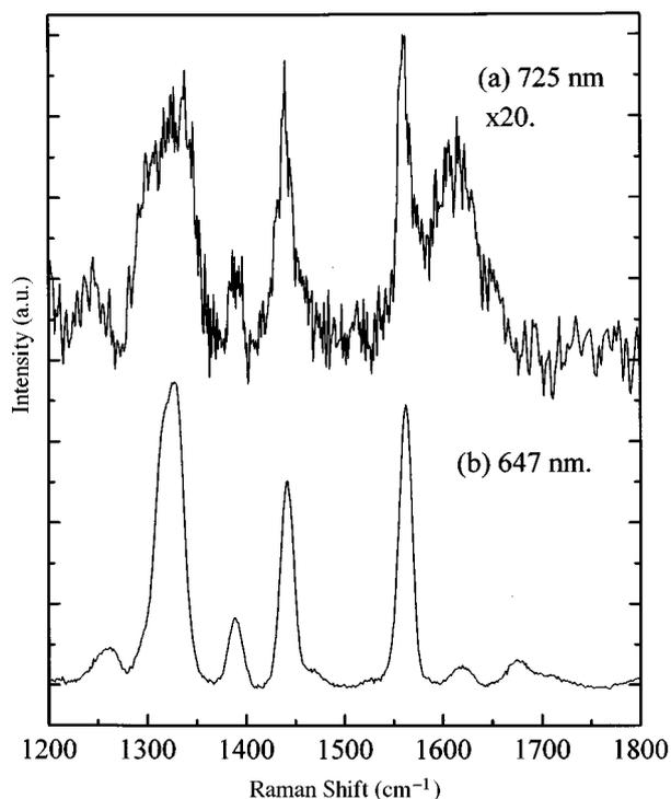
**Fig. 7** Raman spectra of pyromellitic dianhydride adsorbed on Cu(111) excited at 725 nm (a) and 647 nm (b)
