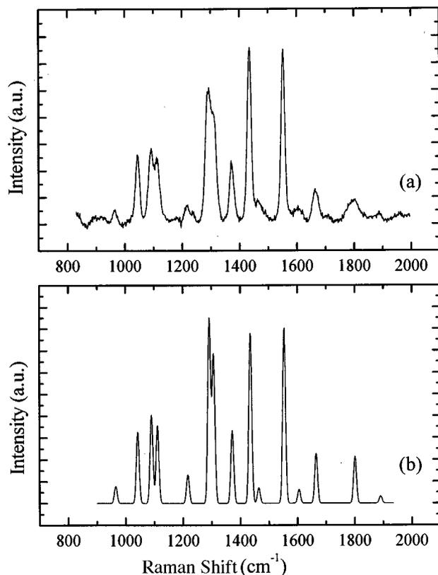
**Fig. 9** Experimental (a) and simulated (b) Raman spectra of pyromellitic dianhydride adsorbed on Cu(100) for 647 nm excitation
