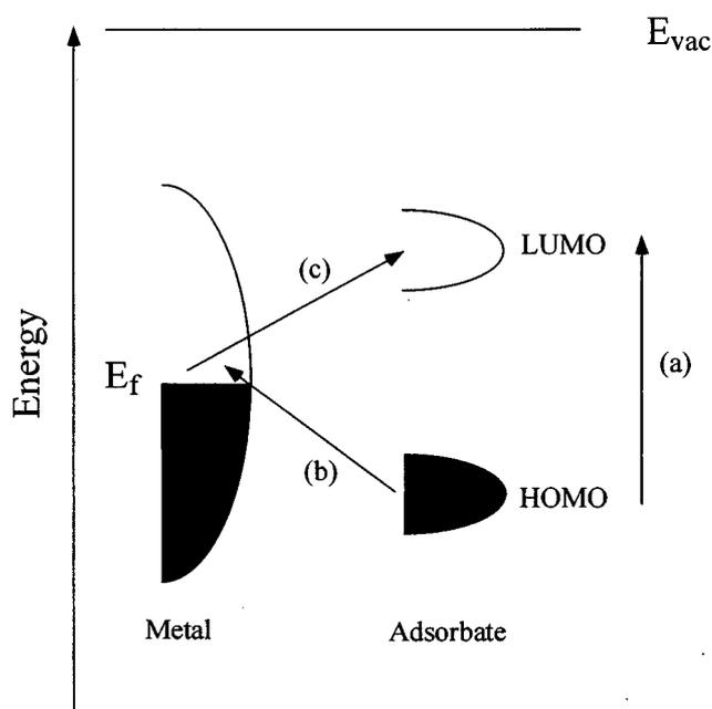
**Fig. 1** Typical energy level diagram for a molecule adsorbed on a metal surface. The occupied and unoccupied molecular orbitals are broadened into resonances by their interaction with the metal states; orbital occupancy is determined by the Fermi energy. Possible charge transfer excitations are shown.
