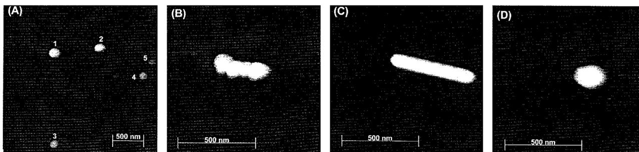
Fig. 2 Tapping mode atomic force microscopy images of selected silver nanoparticles. (A) Particles 1 and 2 showed significant Raman enhancement, the rest did not. (B) A four-particle hot aggregate. (C) A rod-like hot particle. (D) A faceted hot particle. (Reproduced from Ref. 17 by permission).
